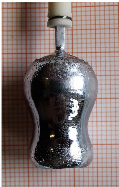
Figure 2: Czocharlski-grown single crystal of \text{FeGa}_{2.85}\text{Ge}_{0.15}
